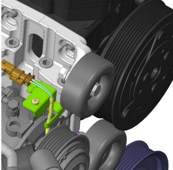
Once the compressor is secured, confirm clearance from the back of the compressor to the EGR body and plug (2011-2016 models only). If it is touching, unbolt the compressor and remove material where necessary to make adequate clearance. The second idler pulley can now be bolted on using the supplied 3/8 bolt, washers, and locknut.
