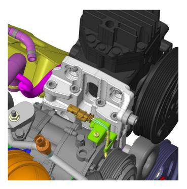
Bolt the compressor to the bracket using **(4)** 3/8 x .875 bolts and medium strength threadlocker into the **TOP** set of holes. You will visually center the compressor front to rear in the slots. Its position can be adjusted later if fine-tuned belt alignment is required. The compressor can now be bolted onto the engine using **(4)** M10x130mm bolts with threadlocker.
