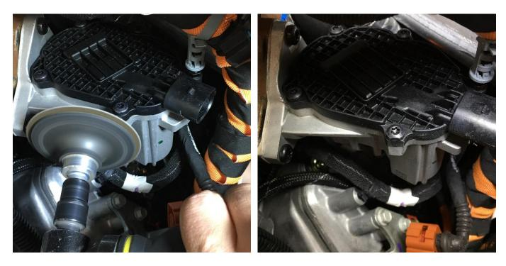
For 2011-2016 models with the factory EGR intact, use a 50-grit sanding pad to flatten the EGR mounting boss as shown.
